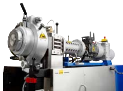
expac® extrusion package: retrofit gear pump to extruder
