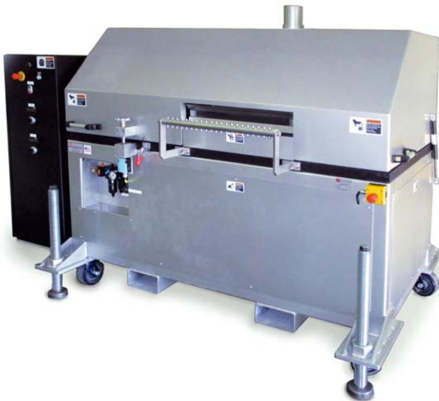
The S3500 Series Strand Pelletizers have been engineered to provide easy, tool-less entry into the stainless steel cutting chamber. The "Slide" Series pelletizers have been designed to substantially reduce maintenance and cleaning time. The front section of the pelletizer is mounted on a linear slide mechanism allowing access into the cutting chamber.
