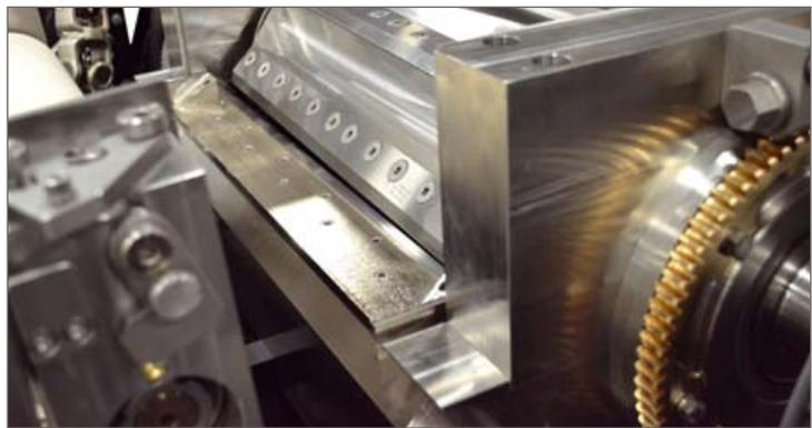
Cutting chamber with Eight blade Pultrusion rotor.
