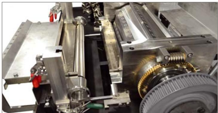
Sliding access to the cutting chamber for easy maintenance.
