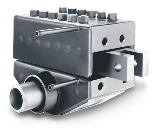
maag pump systems diverter valve is a proven, simple slide-type 3-way valve which allows transfer without disrupting line operation. It is designed for highly viscous fluids.
