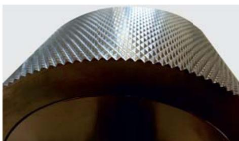
For pelletizing of very abrasive products, like strands filled with glass fibers, we also offer steel feed rolls with wear protective coating.
