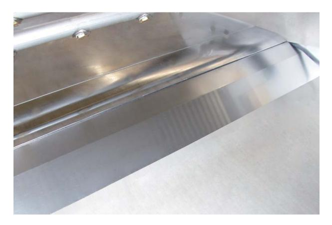
The water guide sheet acts like a bridge from start-up head to strand guide section, neutralizes the height difference and allows a smooth flow of water and strands.
