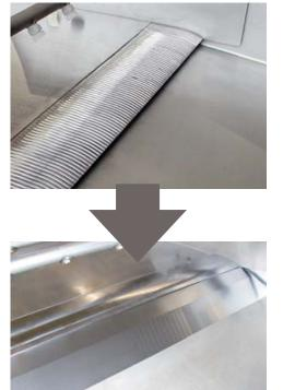
The water guide sheet acts like a bridge from start-up head to strand guide section, neutralizes the height difference and allows a smooth flow of water and strands.
