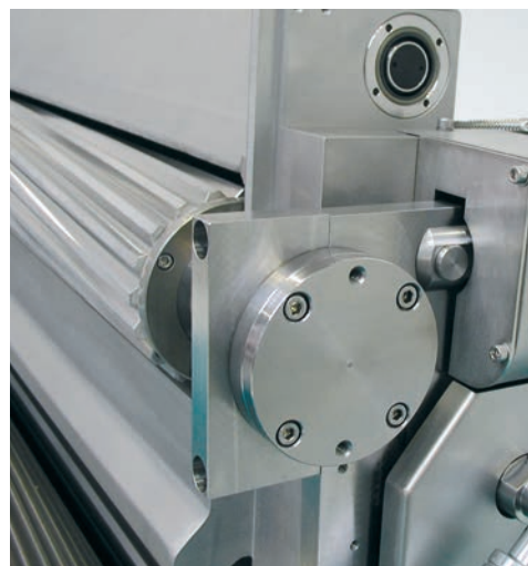
Roller bearing support outside of cutting chamber
