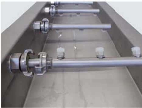
Quick-change spray tubes for simple maintenance during operation
