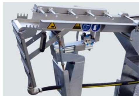
Strand guide section – manually moveable
