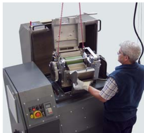
Replacing the cutting head
