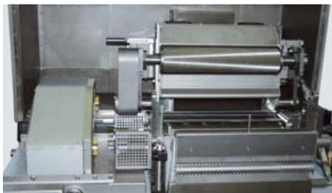
Quick and easy access to all cutting chamber components, without the need for tools
