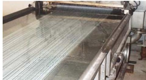
KW 1.400 cooling trough for up to 130 strands
