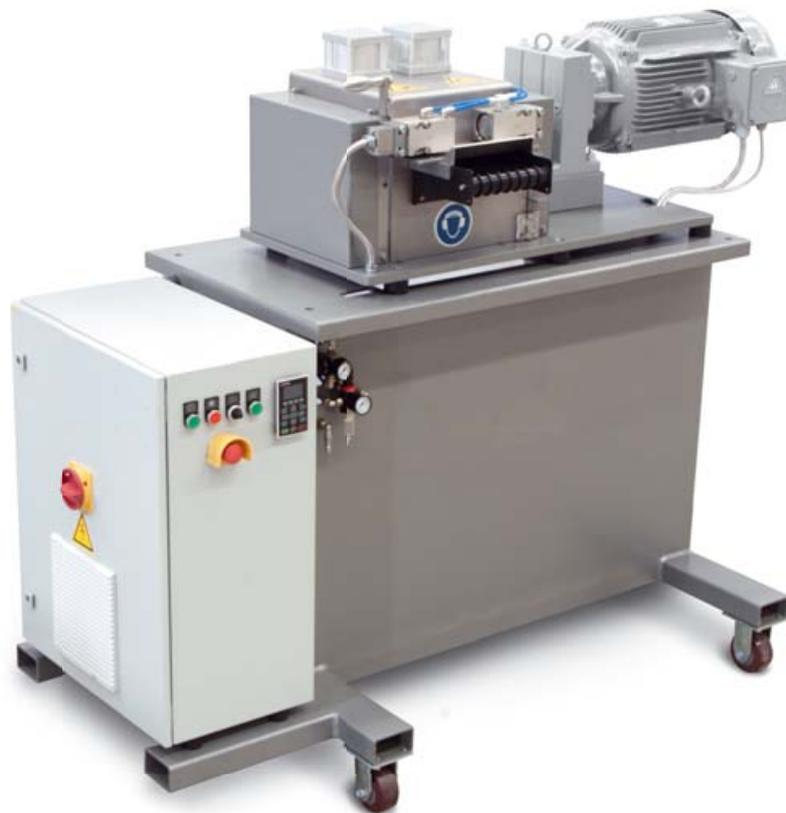
Successfully applied by hundreds of customers in China and abroad, the proven BAOLI strand pelletizers produce the highest quality of cylindrical pellets or micro pellets, ideally suited for further processing. BAOLI is specifically used for strand pelletizing of compounds, blends and masterbatches.
