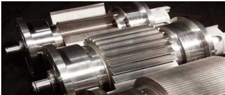
The cutting rotor is the »heart« of every strand pelletizer. The rotor performance is significant for product quality, system availability and production costs.
