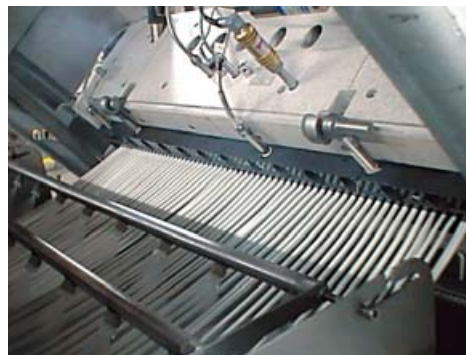
SG 900 die head in operation
