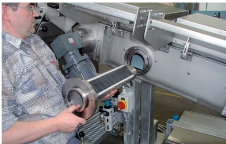
Variable positioning of the exhaust air nozzles
