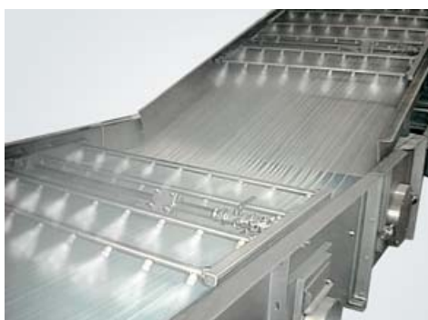
Transition zone from strand guide section to conveyor belt
