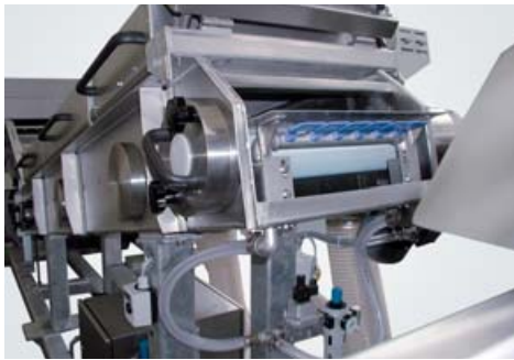
Air nozzles at the transition to the pelletizer
