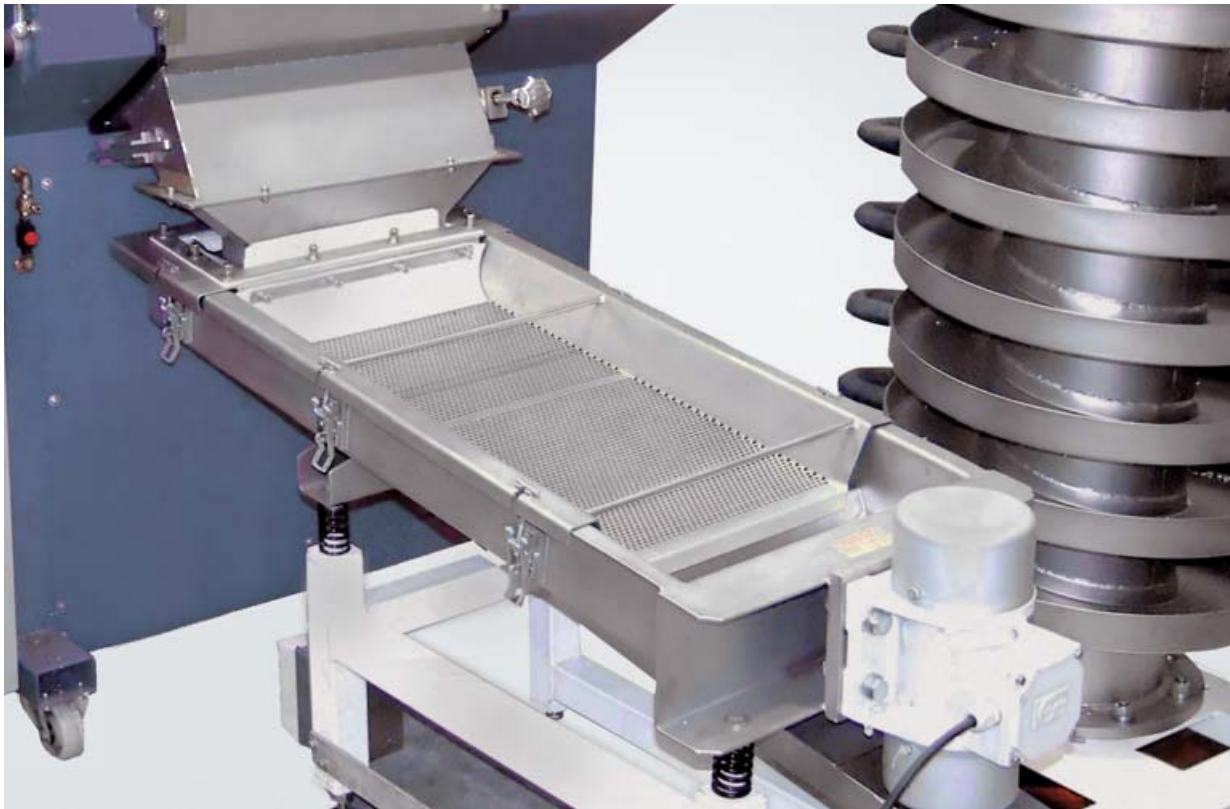
Classifier with spiral conveyor for downstream processing
