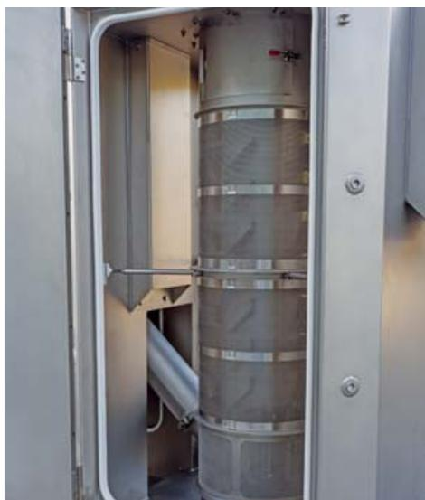
The CYCLO® dryer features double walls filled with insulating material. Sound pressure level of  $\leq 80$  dB(A) is possible. Large, wide doors and larger distances between rotor screens and dryer walls provide easy access to the interior.
