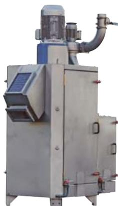
Integration of the intake and air filter into the resin outlet optimizes countercurrent air flow so less air volume is needed for the drying process.
