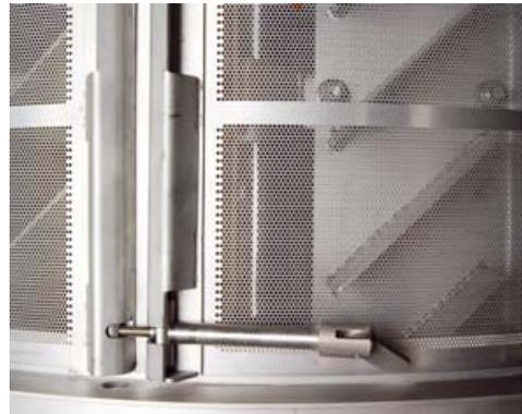
Perforated Screen used for most dryer applications
