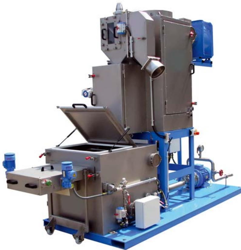
PURO® is an efficient water system technology for any application. The energy-efficient compact systems require minimal space and are suitable for use with both PEARLO® underwater pelletizing systems, M-USG and P-USG underwater strand pelletizing systems. Well thought-out and highly accessible components serve to provide excellent operating characteristics and efficient servicing.
