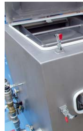
Tempered water system tank with integrated fines removal screen system to remove down to 300 µm particles
