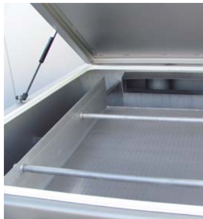
Tempered water system tank with integrated fines removal screen system to remove down to 300 µm particles
