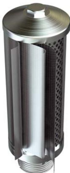
The exchangeable perforated sleeves are made application-specifically from several layers of filter medium, where, depending on the task at hand, and the required filter fineness either screen meshes or metal fiber fleece are used for separation of solids.
