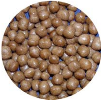
PP Wood Fiber cut with a Gala Pelletizer
