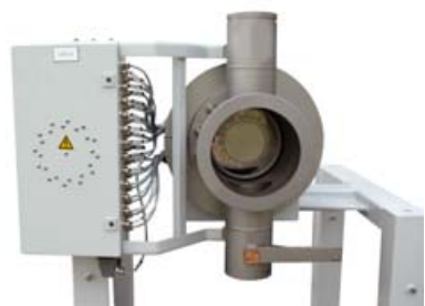
Die Plate heating
