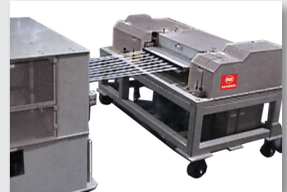
Glass-filled product are feeding into Pultrusion Stand Pelletizer.
