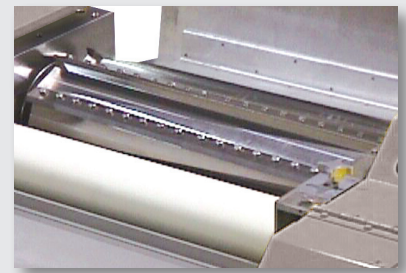
Cutting chamber with eight blade Pultrusion rotor.
