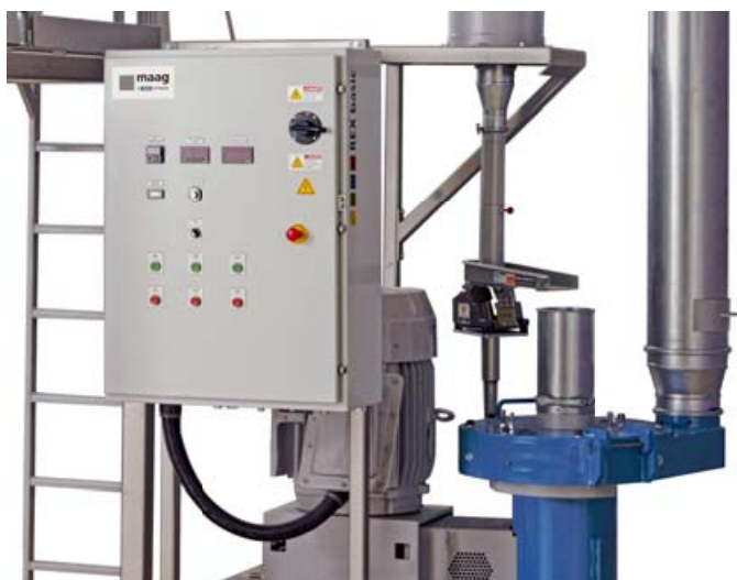
Mill Chamber and Manual Controls
