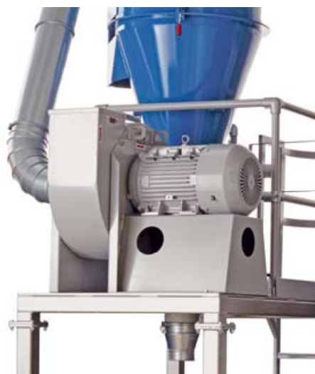
Blower, Cyclone and Transfer System
