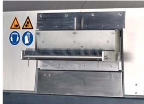
The pellet outlet is also accessible without the use of tools, allowing cleaning work at product changes to be carried out quickly and easily.
