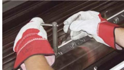
At the cutting rotor, all bolted connections are well covered to prevent undesirable deposits and worn bolt heads. As a result, the life cycle of the cutting tools is significantly increased, and at the same time the scope of cleaning is minimized.
