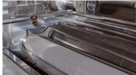
The wide strand inlet with comb guides prevents any overlapping of the strands and keeps the strands in position.
