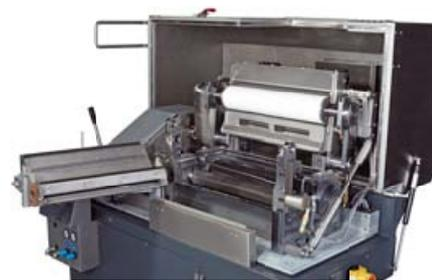
Loose fibers contaminate the pellets, so they are removed from the cutting chamber via the extraction openings before the strands are cut.
