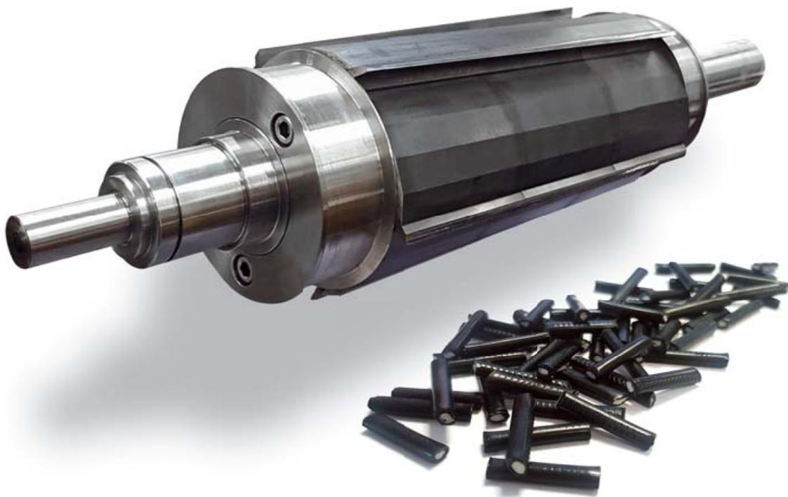
During production of LFT long-fiber pellets using the pultrusion method, fiber strands are drawn continuously through a polymer melt and the individual fibers are embedded in the polymer matrix. After cooling, the resulting fiber/polymer strands are chopped continuously to form pellets. Our LFT rotors fit our PRIMO<sup>PLUS</sup> and M-ASG pelletizing systems.
