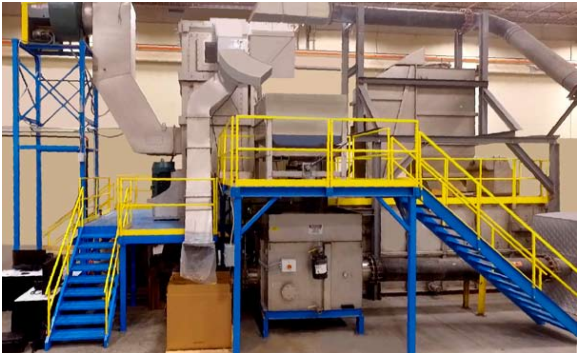
Model 100 High Capacity Centrifugal Pellet Dryer for processing rates up to 150,000 kg/h
